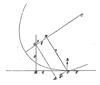
contact. Let GA be that principal axis which lies in the plane PGC and GB the axis at right angles to GA, GC. Let GM be a perpendicular from G on the hori-
